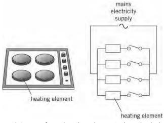
Calculate the resistance of one heating element when the hob is switched on at full power. Give your answer to 2 significant figures.
